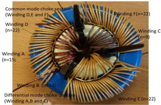
Figure 9 Hybrid magnetic 3 phase EMI filter
