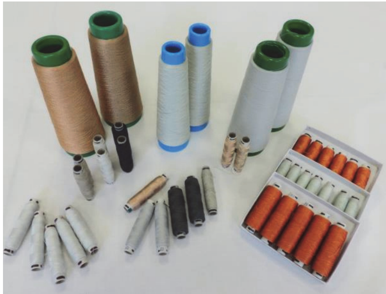
Fig. 2: Hybrid conductive and resistive sewing threads based on metal microwires developed by VUB Company in close collaboration with UWB.
