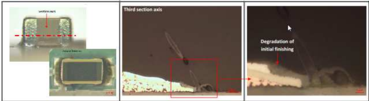
Fig6: The extremity of the termination evidenced Tin over Nickel and Copper. Tin is partially oxidized (grey color) like whiskers. In the section plan the tubular shape is evidenced. Whiskers growth is on the ceramic nearby or in contact with the Tin edge of Tin layer.
