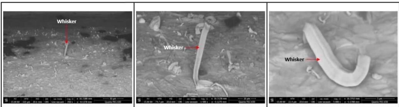
Fig3: The shape of “standard” Whiskers was observed on another component terminal and compared with those found on the MLCCs.
