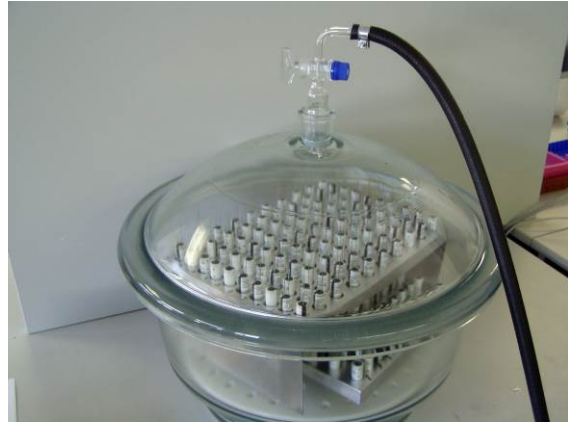
Fig. 3. EGGO supercapacitors screening facilities - burn-in (left) and vacuum (right)
