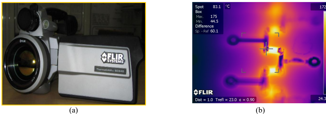
Fig. 14. a) Thermography camera SC640, b) IR Picture of self-heated resistors.
