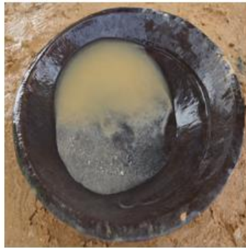
Example of simple washing process at an artisanal mine
