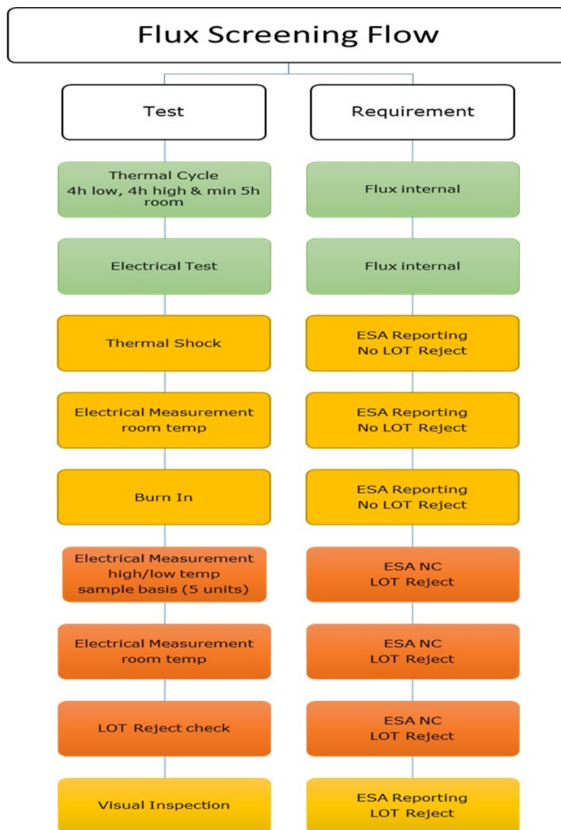
Fig. 3. The flow of pre-screening (Flux internal) and formal Screening (ESCC reporting and LOT reject apply)
