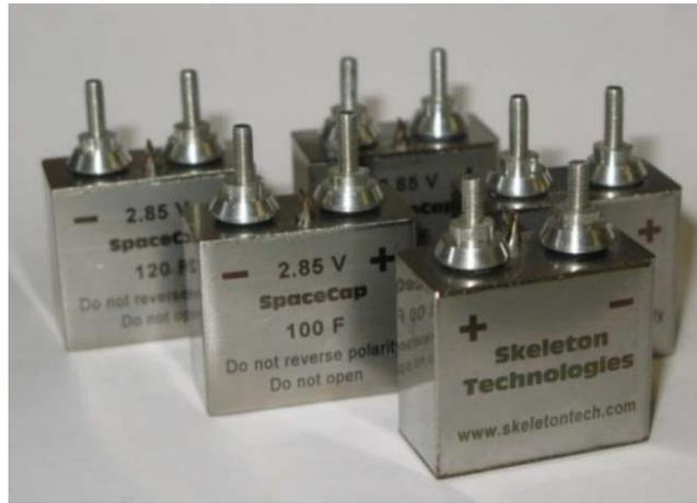
*Fig.1. Completed SpaceCap prototypes*
