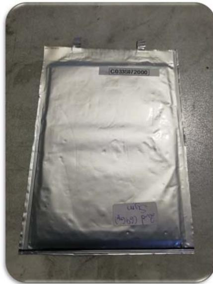
*Fig.2. Graphene-enabled supercapacitor pouch*
