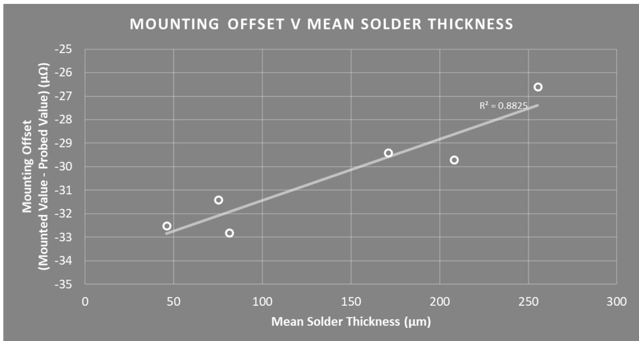
Figure 15 Correlation between Mean Solder Thickness beneath Terminations and Mounting Offset for LRMAP2512-R0005FT4
