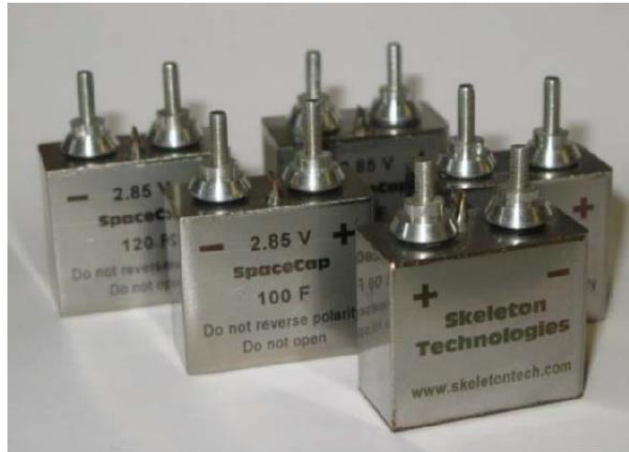
Figure 3: SpaceCap supercapacitors prototypes.
