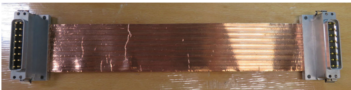
Fig. 8. Picture of a harness composed by a shielded FFC pair and 2 16way FFC Versatys connectors
