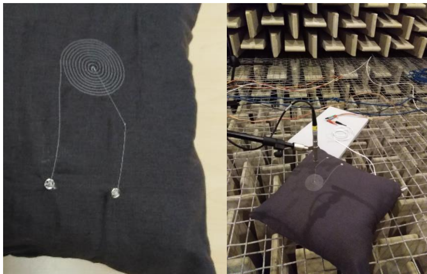
Fig. 7 Textile speaker embroidered in a pillow and measurement setup
