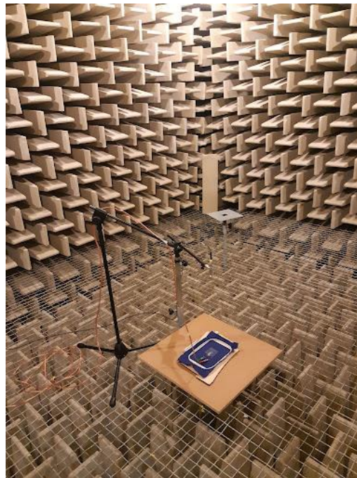
Fig. 4 Sample measurement setup in an anechoic chambre
