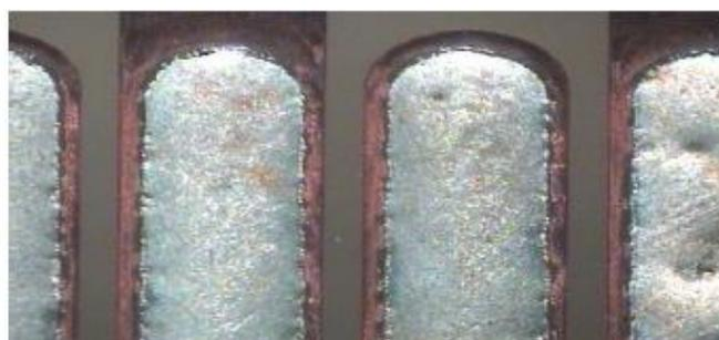
Fig. 25: uncovered solder joints
