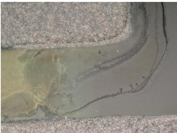
*Fig.7 Precipitates caused by leakage current*
