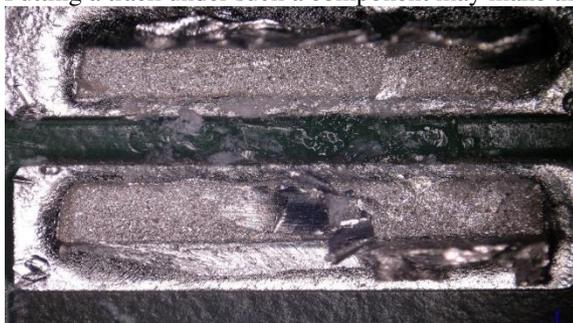
Fig 22. The gap with residues under the reverse geometry chip.
