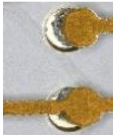
Fig.31. BGA 1020 after cleaning
