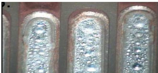
Fig. 24 Solder joints covered by glass
