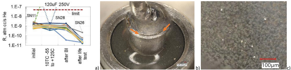
Fig.10. Variation of hermeticity in lot 1 of 120\ \mu\text{F} 250\ \text{V} aluminum capacitors during testing before HTS (a), a crack between solder and the tube in SN28 (b), and a close-up view of the glass seal in capacitors showing multiple bubbles inside and at the surface of the glass (c).
